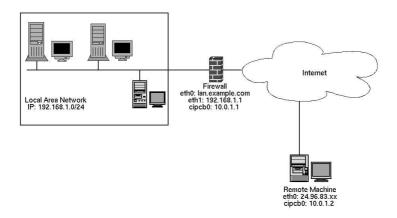
Figure 6-2. Typical CIPE Server and Client Configuration
