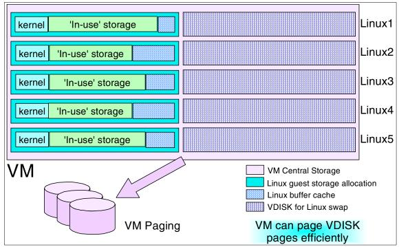
Figure 3-5 Linux swap using VDISK
