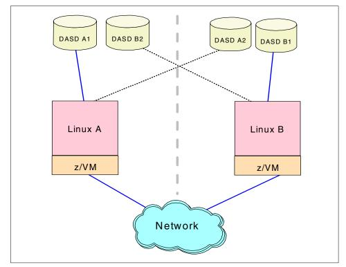
Figure 7-3 Network block device cross-site
