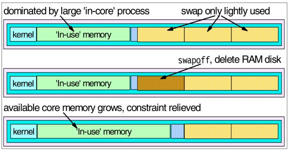
Figure 3-7 Relieving memory constraint in RAMdisk swap configuration
