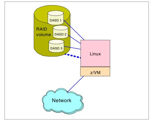
Figure 7-2 Software RAID example
