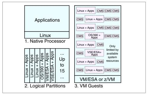
Figure 1-1 Linux for zSeries and S/390 operation modes
