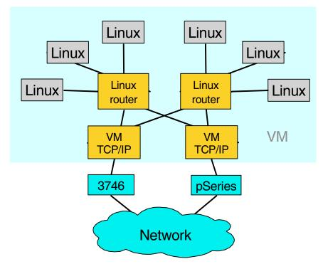
Figure 3-12 Combining VM TCP/IP and Linux virtual routing
