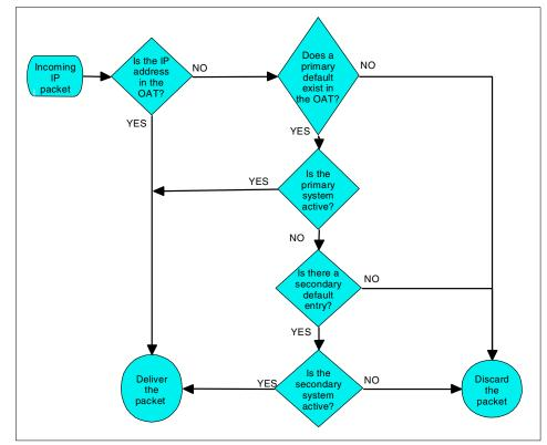
Figure 4-8 Packet path through the OSA
