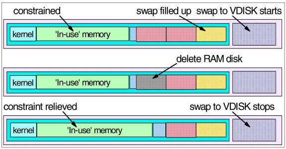
Figure 3-9 Relieving memory constraint in hybrid swap configuration
