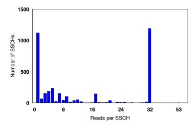
Figure 8-2 Number of Read-CCWs in a channel program
