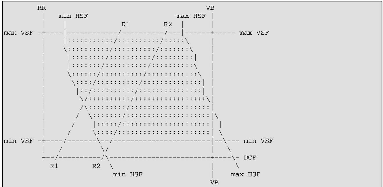
This is a generic monitor mode diagram. The x axis of the diagram shows the clock rate (DCF), the y axis represents the refresh rate (RR). The filled region of the diagram describes the monitor's capabilities: every point within this region is a possible video mode.
