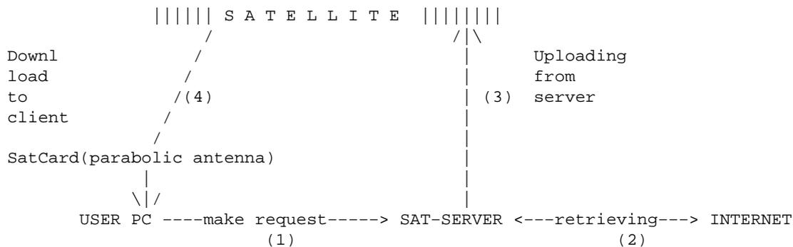
So first we make the request (1) (using our Internet connection) to the Sat-Server, after it will retrieve out info from Internet (2) and it will send it to Satellite (3); in the end we would receive data from the it (4) to our home using a parabolic antenna and a Sat Card.
