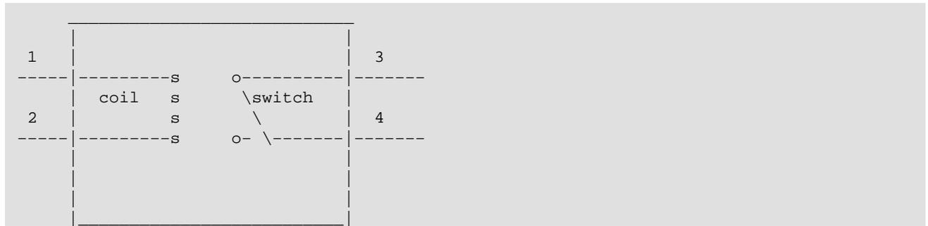
In the diagram above, pin 3 and pin 4 are disconnected by default. When you send +12V between pin 1 and pin 2, it will turn on a switch, and pin 3 and 4 are now connected.
