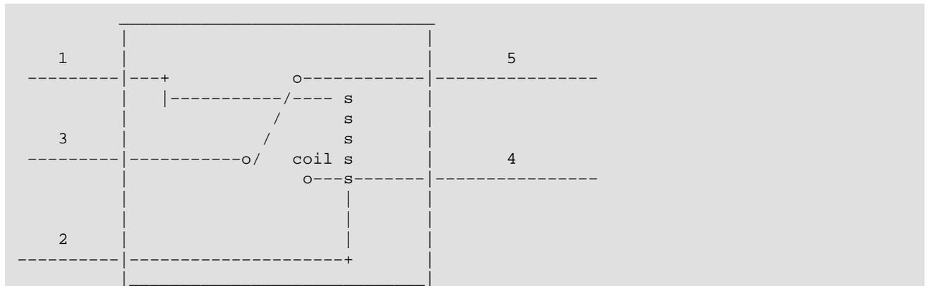
In the above diagram pin 3 is connected to pin 5, by default. By sending +12V between pin 1 and pin 2, you will turn on a switch. Pin 1 and pin 2 will disconnect, and pin 5 and pin 4 will connect.
