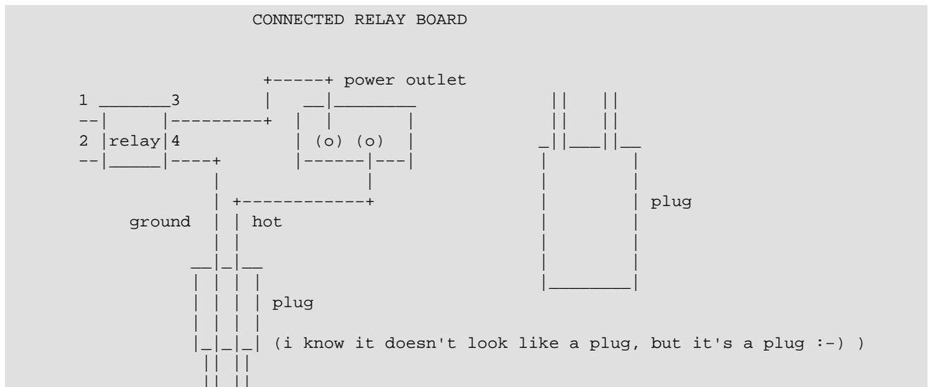
To connect the system, just connect your home electrical device to the power outlet. That is it! You don't need to make any change on the electrical device. And you can connect any kind of device to that power outlet. Plug this power outlet into any wall outlet.
