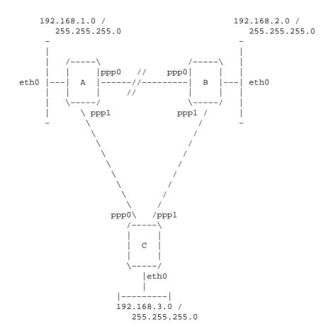
We have three routers A, B and C. Each supports one ethernet segment with a Class C IP network (netmask 255.255.255.0). Each router also has a PPP link to each of the other routers. The network forms a triangle.
