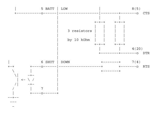
NOTE!!!: Shutdown pins in the tech info supplied with UPS (4 and 6) are given incorrectly! The valid ones are 6 and 7, as shown above. Note2: Pin numbers on the PC side in the brackets are for 25-pin connector, outside - for 9-pin one.
