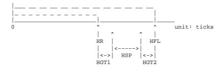
Now, we would like to place a sync pulse of length HSP as shown above, ie, between the end of clock ticks for display data and the end of clock ticks for the entire frame. Why so? because if we can achieve this, then your screen image won't shift to the right or to the left. It will be where it supposed to be on the screen, covering squarely the monitor's viewable area.
