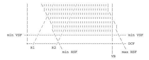
This is a generic monitor mode diagram. The x axis of the diagram shows the clock rate (DCF), the y axis represents the refresh rate (RR). The filled region of the diagram describes the monitor's capabilities: every point within this region is a possible video mode.
